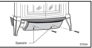
Fig. 15 Use spacers and screws to position the ashdoor heat shield.
